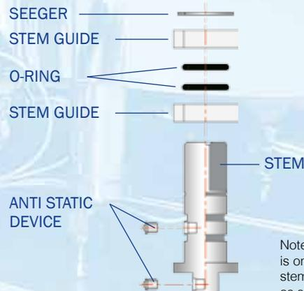
Note: Anti-static device for 1/2"-3/4" is on the side and bottom of the stem. For other sizes, is located as shown in the drawing.
