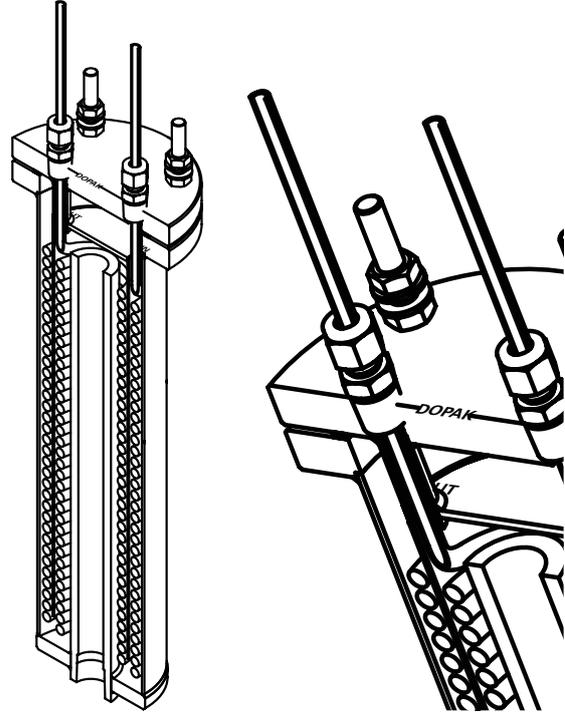
The Dopak double coil, bucket type sample cooler is an effective and efficient heat exchanger where higher flow is required. Standard tube side material is SS316/316(L). Other material is available on request.
